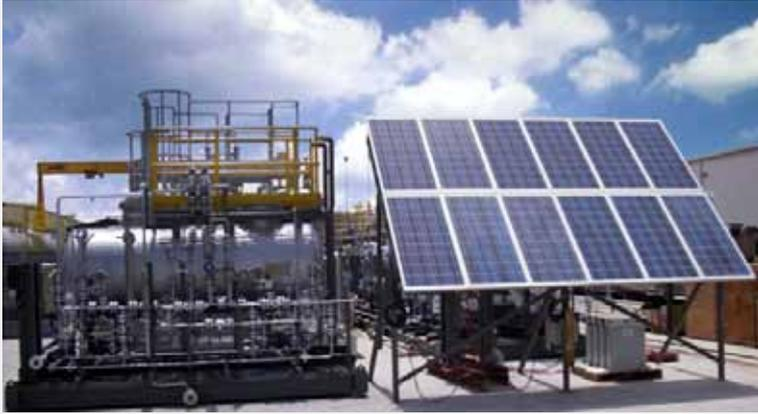
Chemical injection skids are used for injecting a specific and precise quantity of chemical into a system at a required pressure and are in use in Oil & Gas applications. Solar PV Systems are the ideal power source for driving the pump of the skids in remote locations. The solar PV system is equipped with a battery bank to provide power in terms of low sun hours. These systems are well designed to operate in hazardous regions.
